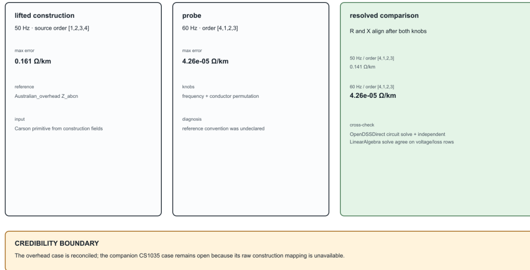
Figure 20.2: The overhead mismatch is reconciled by frequency and conductor-order probes, while the independent CS1035 matrix remains outside the reproduced model.
